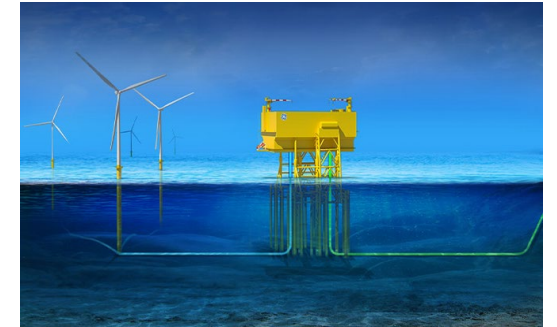
High Voltage Direct Current (HVDC)
