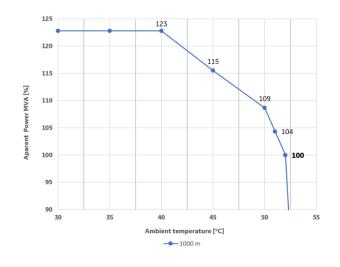
Applicable for grid voltage ≥ nominal voltage, altitudes >1000m on request 13.
