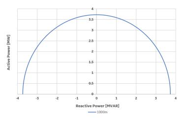
14. PQ diagram for LV5+ 1566 at nominal grid voltage, 1300 Vdc and 40  $^\circ$ C ambient
