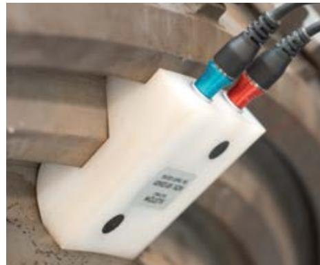
Design specific Eddy Current probe – inspection of turbine radial grooves
