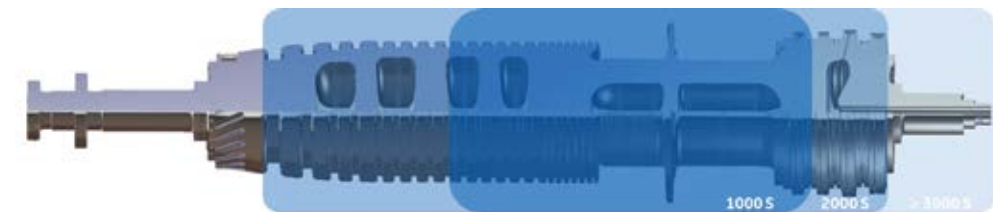
GT24/GT26 indicative inspection schedule based on number of starts
