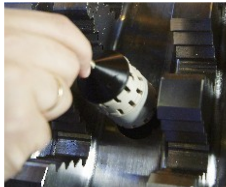
Eddy Current testing of radial bore hole
