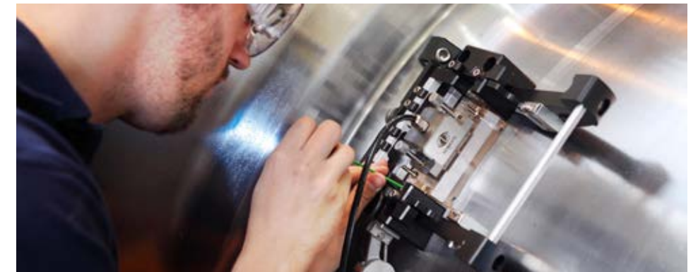
NDT specialists with cooling cavity scanner
