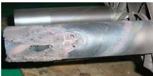
FIGURE 18: Gas turbine fuel nozzle damage from a flame holding event
