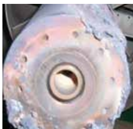
FIGURE 18: Gas turbine fuel nozzle damage from a flame holding event
