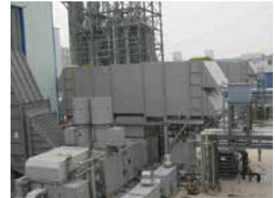
FIGURE 13: A: Frame 9E.03 operating on steel mill gases at a plant in China; B: LM2500+ operating on high H 2 coke oven gas
