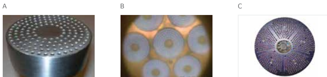
FIGURE 10: A: multi-tube mixer concept hardware, B: combustor test of multi-tube mixers on a H_2/N_2 fuel blend, and C: commercial configuration of the DLN 2.6e combustor
