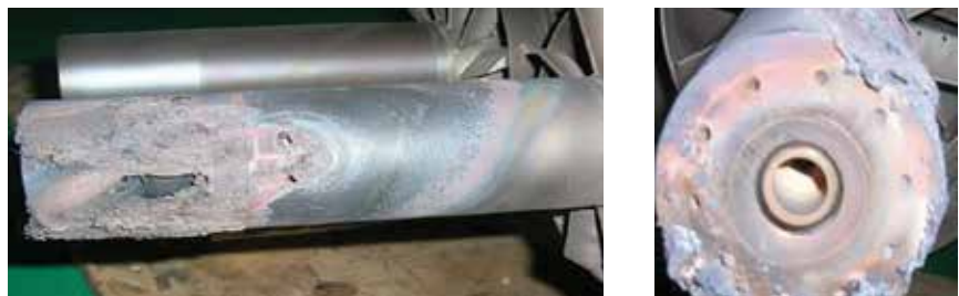
FIGURE 18: Gas turbine fuel nozzle damage from a flame holding event
