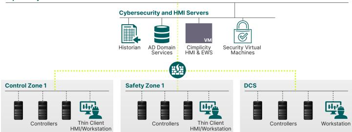
GE Vernova's cybersecurity platform features a broad range of capabilities and offers efficient integration in OT environments. (Network configuration is only an example – configuration and implementation may vary.)
