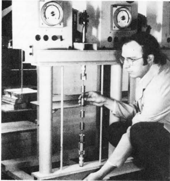
Figure 10. Apparatus used for dead weight load testing.
