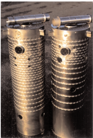
Figure 19. Louvered low NO x lean head end combustion liners
