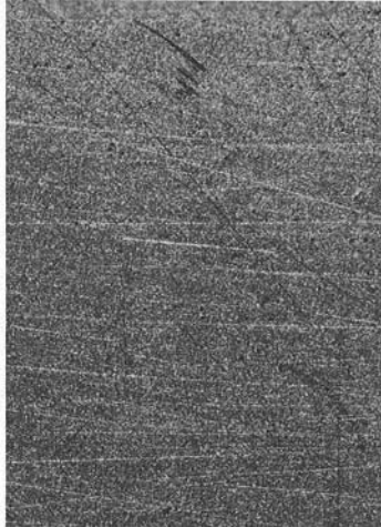
Figure 8. Fine black spots are corrosion pits which developed during 3000 hr of exposure. (Scratches were present prior to testing.)
