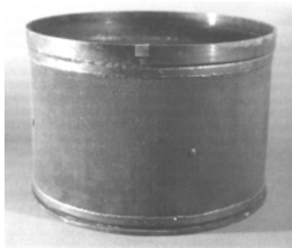
Figure 4. TBG COGEN strainer.
