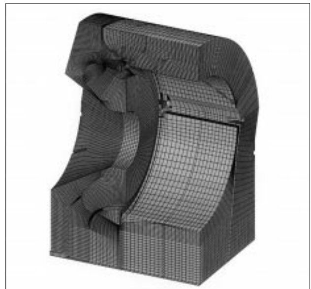
Figure 31. Calculation grid for exhaust hood CFD analysis
