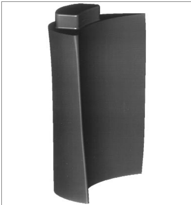
Figure 65. Solid model of typical bucket designed by TADS
