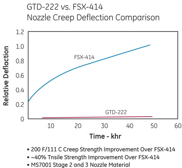
Figure 57. GTD-222+ vs. FSX-414 nozzle creep deflection comparison.
