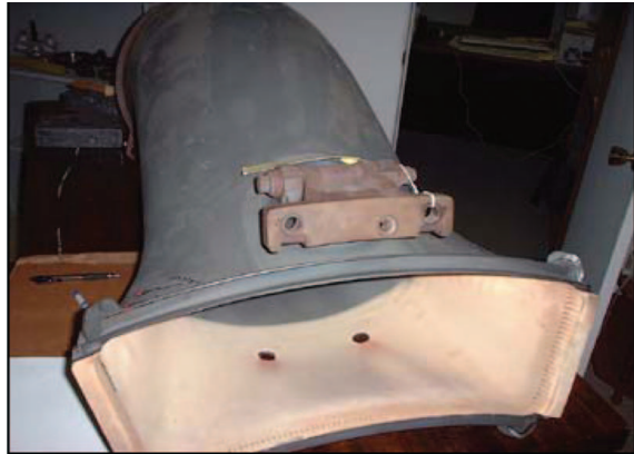
Figure 41. Full Nimonic 263™ transition piece with cloth seals.
