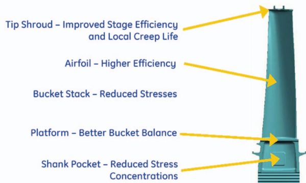
Figure 59. New stage 3 bucket design.
