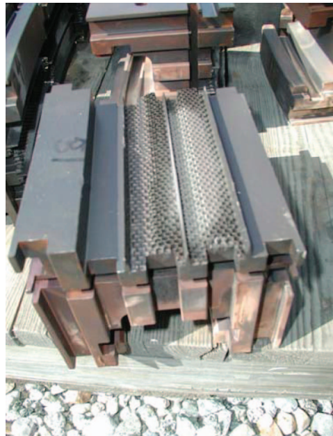
Figure 80. Shroud block with honeycomb sealing.
