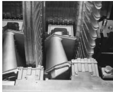
Figure 78. Stage 2 and three hot gas path showing shroud blocks.
