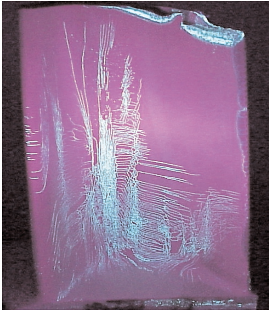
Figure 1. Stress cracked bucket
