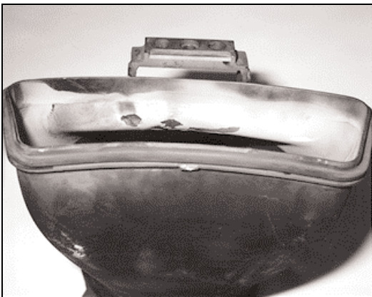
Figure 31. Turbine run transition piece with manually-applied TBC (8,000 hours)
