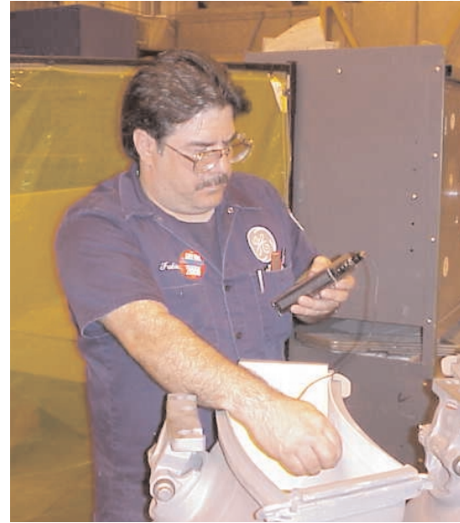
Figure 20. Non-destructive thickness survey for TBC on transition pieces
