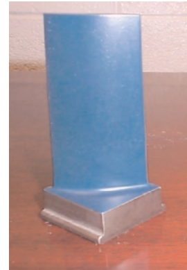
Figure 25. Compressor airfoil coated with GECC-1
