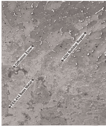
Figure 8. Metallurgical evaluation of ADH repair on FSX-414
