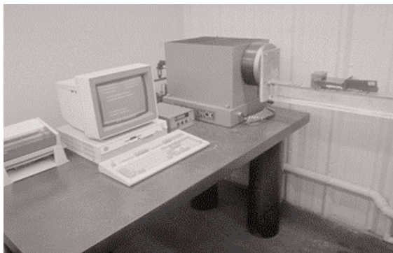
Figure 18. Bucket weighing and charting equipment
