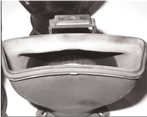
Figure 30. Turbine run transition piece with robotically-applied TBC (8,000 hours)
