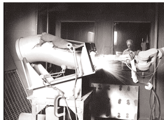
Figure 26. Robotic application of TBC on MS7001E transition piece
