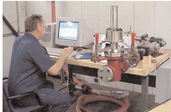
Figure 24. Fuel nozzle air flow test machine
