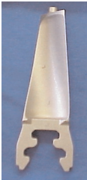
Figure 7. Tangential entry “Pinetree” dovetail bucket
