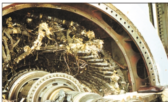
Figure 15. Catastrophic retaining ring failure
