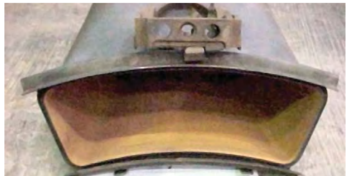
Figure 44. Nimonic™ transition piece showing downstream end coated with TBC
