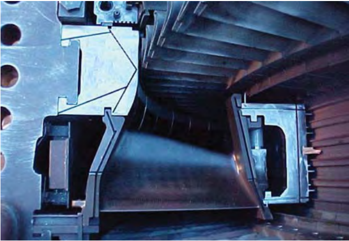
Figure 99a. Installed interstage brush seal
