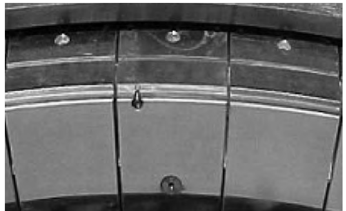
Figure 94. Stage 1 shrouds coated with abradable coating
