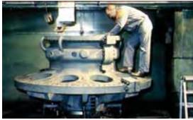
Figure 19. 13th compressor stage extraction for stage 2 nozzle cooling
