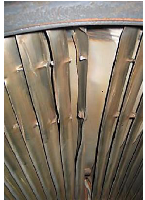
Figure 6 – Turbine bucket damage from torsional resonance
