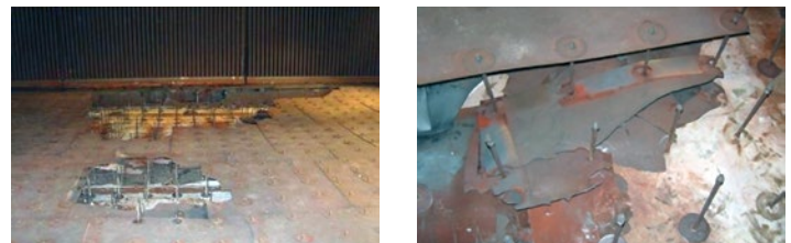
Figure 2: Damage liner plate and stud bolt from GT strong flow and pulsation
