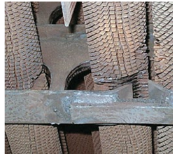
Figure 1: Fin wear from friction with damaged restraint
