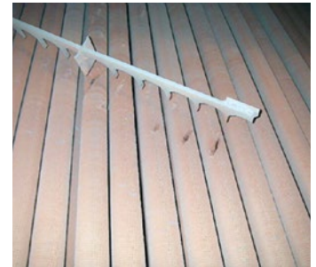
Figure 1: Fin wear from friction with damaged restraint
