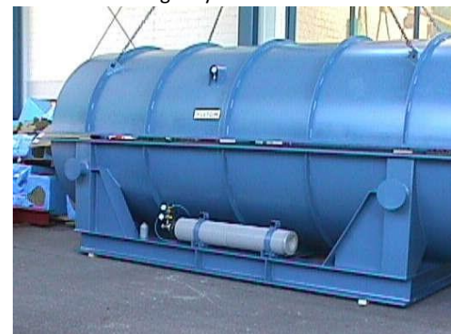
Figure 40: Nitrogen purged transformer furnished with gas cylinder
