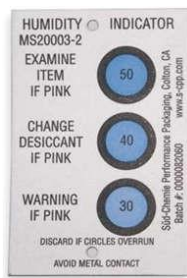
Figure 32: Humidity indicator card
