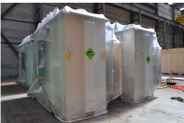
Figure 40: Nitrogen purged transformer furnished with gas
