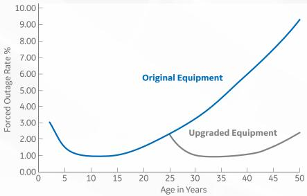
An industrial steam turbine experiences performance deterioration over time. The rate of the deterioration is influenced by the turbine design, the steam quality, and the way the turbine is operated.
