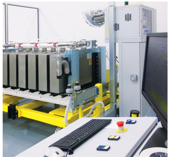
VSC module end of line production test
