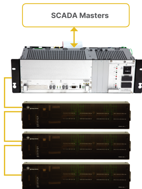
Figure 1: Simple architecture of I/O modules communicating to the D20 RTU
