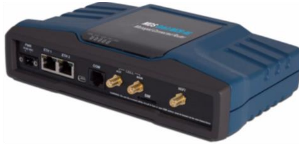
Figure 1-1. MCR-4G Unit (Standard 2E1S configuration shown)
