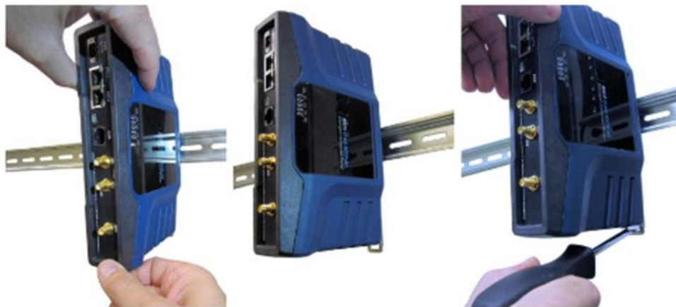
Figure 2-14. DIN Rail Attachment and Removal (Pull down tab to release from rail)
