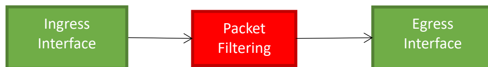
Figure 3-154. Packets Being Forwarded Through the Unit
