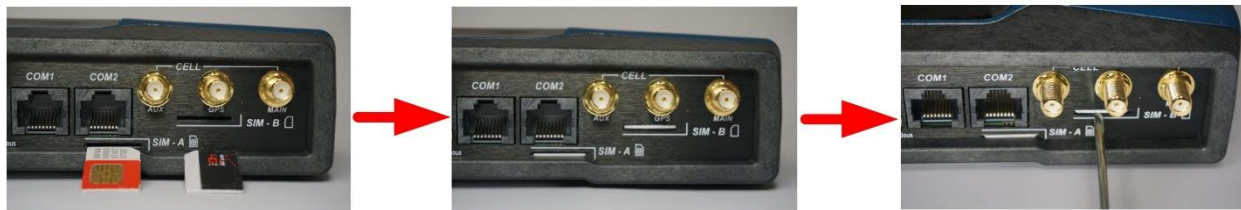
Figure 3-24. Steps for Inserting SIM Cards on ECR and MCR with diagonal alignment
