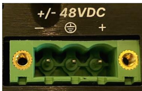
Figure 2-8. Connector configuration for 3-conductor models
