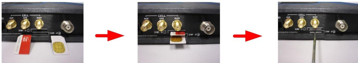
Figure 3-23. Steps for Inserting SIM Cards on MCR with horizontal alignment
