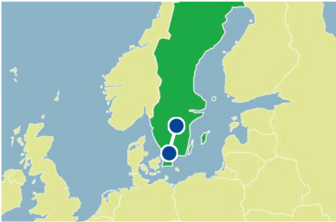
250 km long DC connection, combining overhead lines and underground cable, between Barkeryd and Hurva
