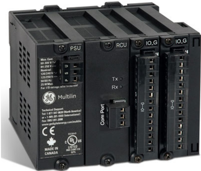
Figure 2-26: RMIO unit showing 2 IO_G modules
