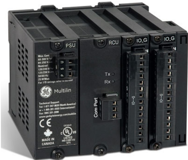
Figure 2-21: RMIO unit showing 2 IO_G modules
