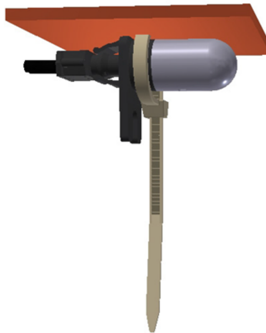
Figure 2-18: AF point sensor, cable tie mount
