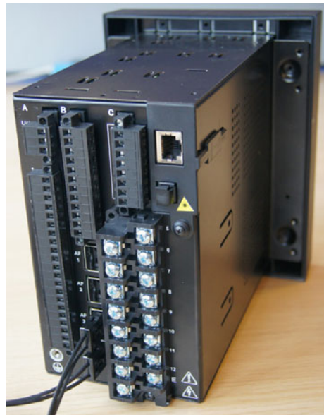
Figure 2-20: AF point sensors connected to 350 relay
