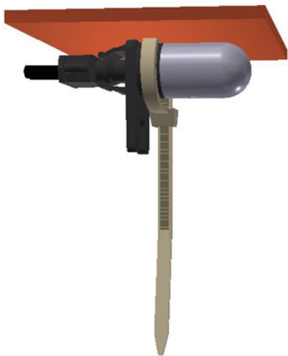
Figure 28: AF point sensor, cable tie mount
