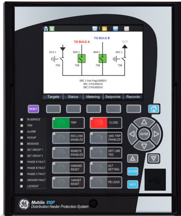
Figure 64: 10-pushbutton membrane front panel
