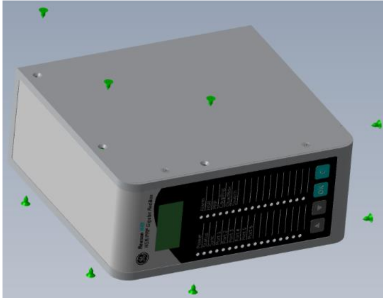
Figure 75: Reason H49 – Location of M6 Screws to be removed
