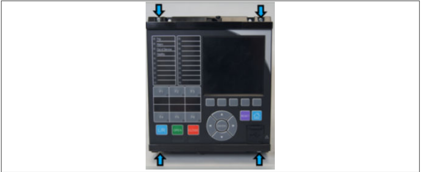
Figure 213: 30TE (without cam) screws placement
