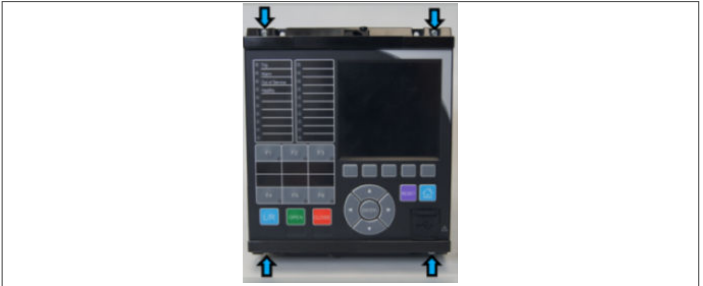
Figure 216: 30TE (with cam) screws and cams placement
