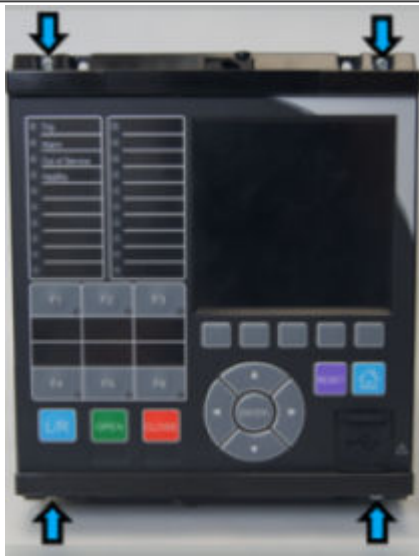
Figure 194: 30TE (without cam) screws placement
