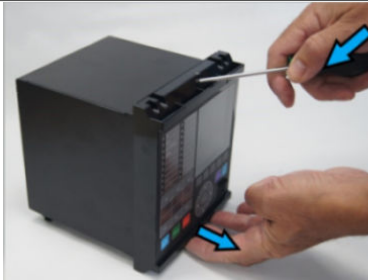
Figure 201: 30TE 1 lever rotation, direction and extraction
