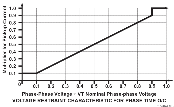
Figure 269: Phase time overcurrent voltage restraint characteristic
