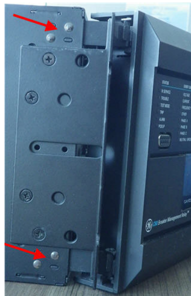
Figure 8-20: Unscrew basic front panel mounting bracket on left side (note riveted hinges with red arrows)
