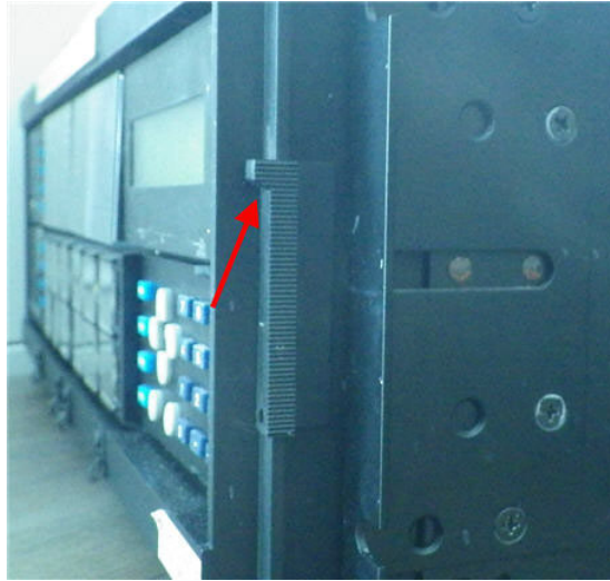
Figure 8-15: Lift latch on basic front panel to open
