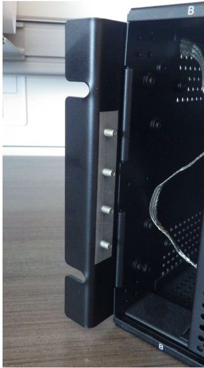
Figure 8-21: Attach mounting bracket on left side (enhanced front panel shown; no power supply module in first slot)
