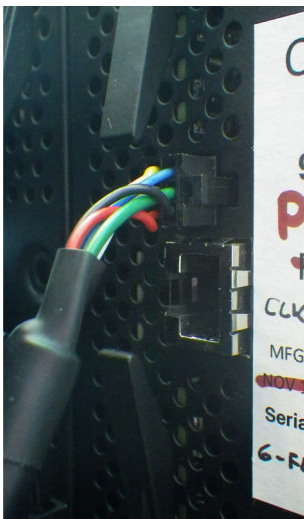
Figure 8-26: Connect graphical front panel to top connection on CPU module
