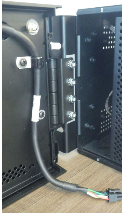
Figure 8-23: Attach to left mounting bracket inside relay
