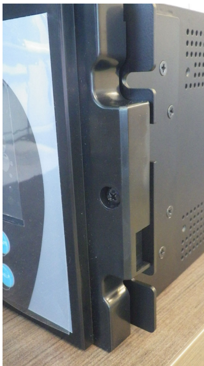
Figure 8-27: Screw to attach graphical front panel to mounting bracket
