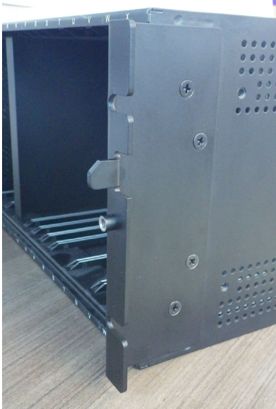
Figure 8-22: Attach mounting bracket to relay on right side
