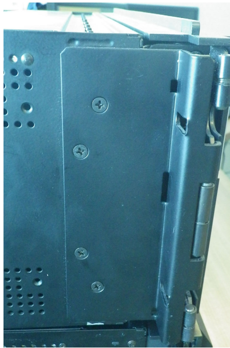
Figure 8-20: Unscrew basic front panel mounting bracket on left side (note riveted hinges with red arrows)
