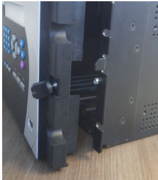
Figure 8-16: Remove enhanced front panel mounting bracket on right side
