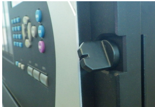
Figure 8-14: Loosen thumb screw on enhanced front panel to open
