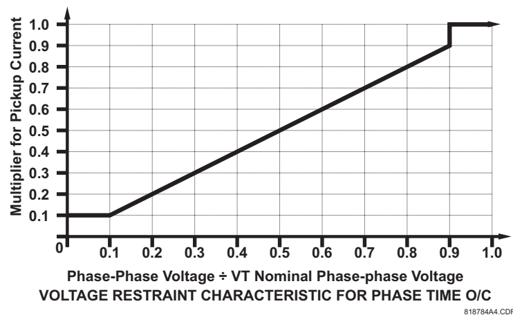
Figure 5-111: Phase time overcurrent voltage restraint characteristic
