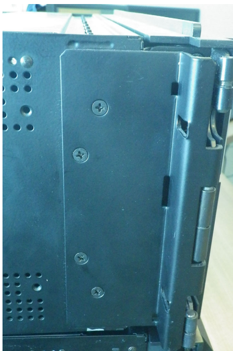
Figure 10-19: Unscrew enhanced front panel mounting bracket on left side
