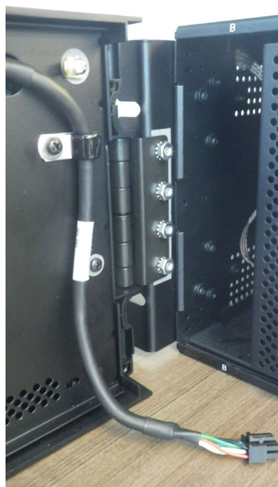
Figure 10-23: Attach to left mounting bracket inside relay
