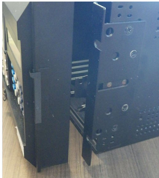
Figure 10-17: Remove basic front panel mounting bracket on right side
