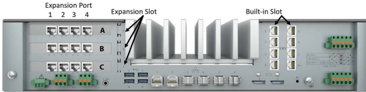
Figure 3: G500 rear view with UART and expansion slots
