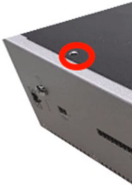
Figure 2-2: Back view of G100 with suggested security seal location
