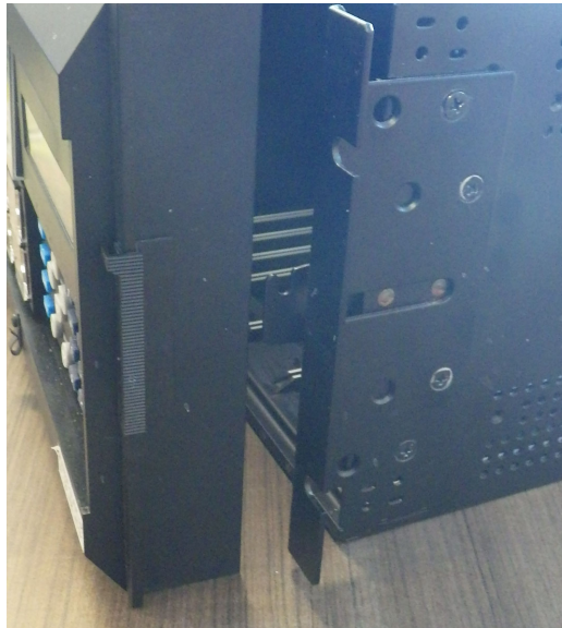
Figure 11-17: Remove basic front panel mounting bracket on right side
