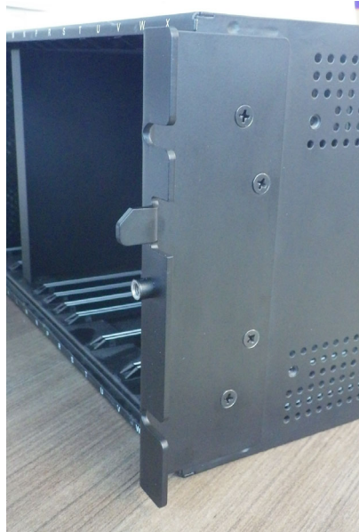
Figure 11-22: Attach mounting bracket to relay on right side
