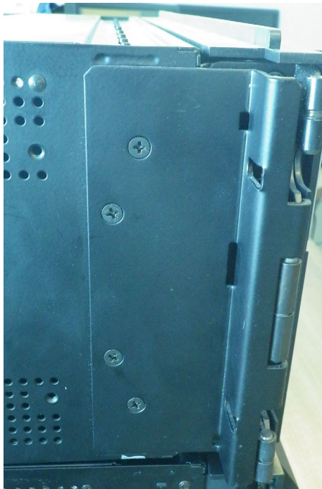
Figure 11-19: Unscrew enhanced front panel mounting bracket on left side
