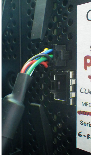
Figure 11-26: Connect graphical front panel to top connection on CPU module
