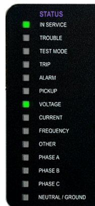
Figure 4-52: Example of LEDs on graphical front panel
