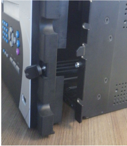
Figure 11-17: Remove basic front panel mounting bracket on right side
