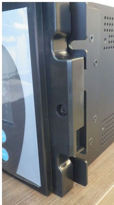
Figure 10-27: Screw to attach graphical front panel to mounting bracket
