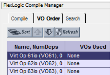
Figure 4-83: Ordering FlexLogic entries
