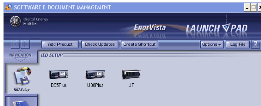
Figure 3-64: UR device added to Launchpad window
