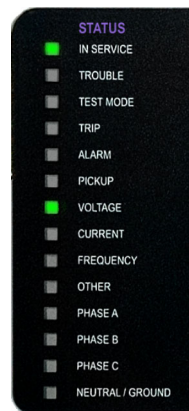
Figure 4-52: Example of LEDs on graphical front panel
