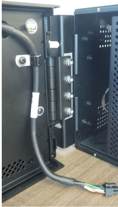
Figure 10-23: Attach to left mounting bracket inside relay
