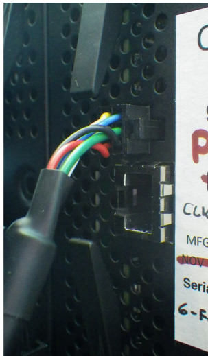
Figure 10-26: Connect graphical front panel to top connection on CPU module
