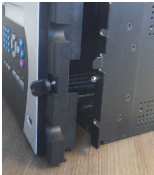
Figure 10-16: Remove enhanced front panel mounting bracket on right side
