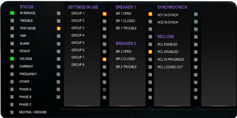
Figure 4-48: Typical LED panel for enhanced front panel
