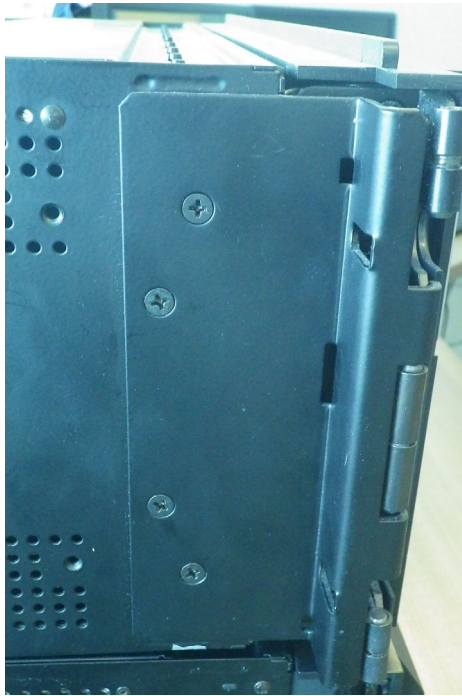
Figure 10-20: Unscrew basic front panel mounting bracket on left side (note riveted hinges with red arrows)
