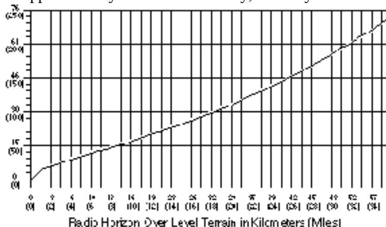
Figure 9-2. Antenna Height vs. Theoretical Radio Horizon
