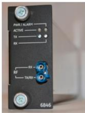
Figure 6-8. LN Radio Module (Part No. 03-6846A01-Lxx)
