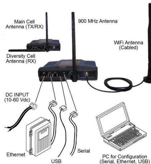
Figure 2: Typical MCR installation (equipment images may differ)
