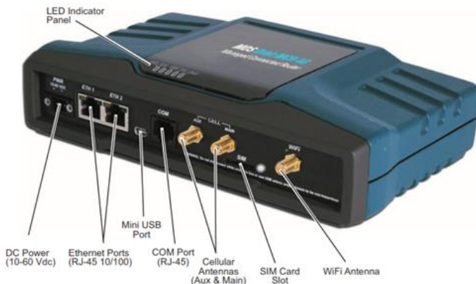
Figure 1: MCR Sample Unit, Showing Connectors & Indicators
