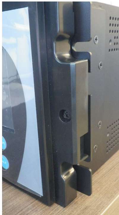
Figure 9-27: Screw to attach graphical front panel to mounting bracket
