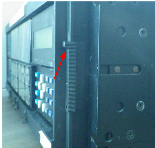
Figure 9-15: Lift latch on basic front panel to open
