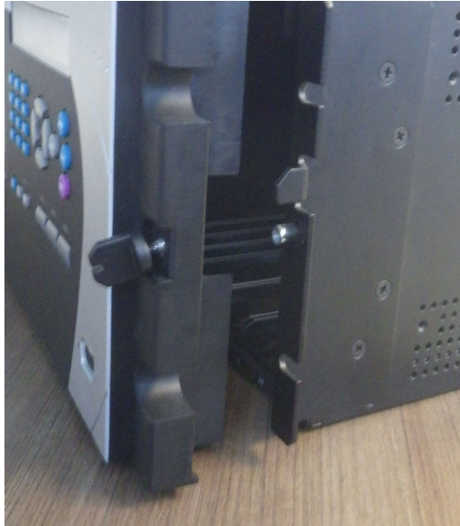
Figure 9-17: Remove basic front panel mounting bracket on right side
