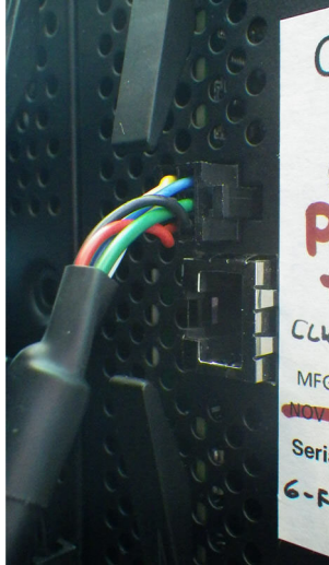
Figure 9-26: Connect graphical front panel to top connection on CPU module
