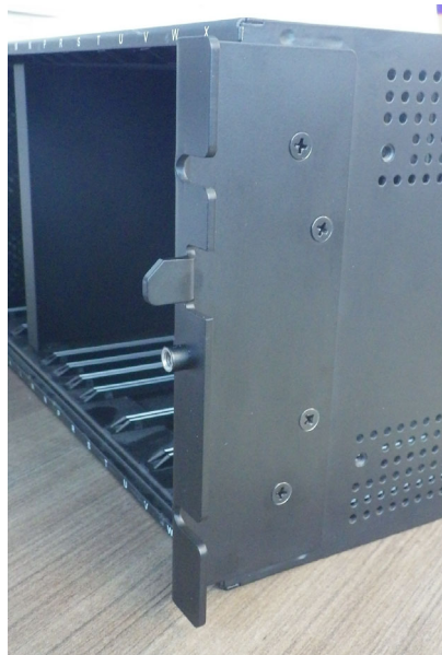
Figure 9-22: Attach mounting bracket to relay on right side
