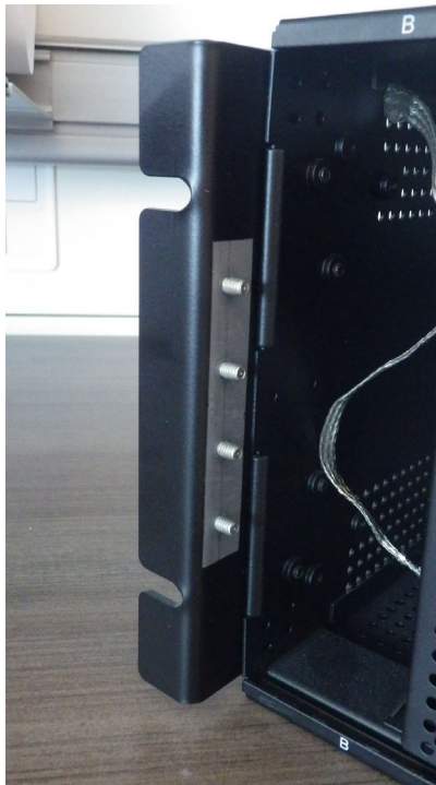
Figure 9-21: Attach mounting bracket on left side (enhanced front panel shown; no power supply module in first slot)
