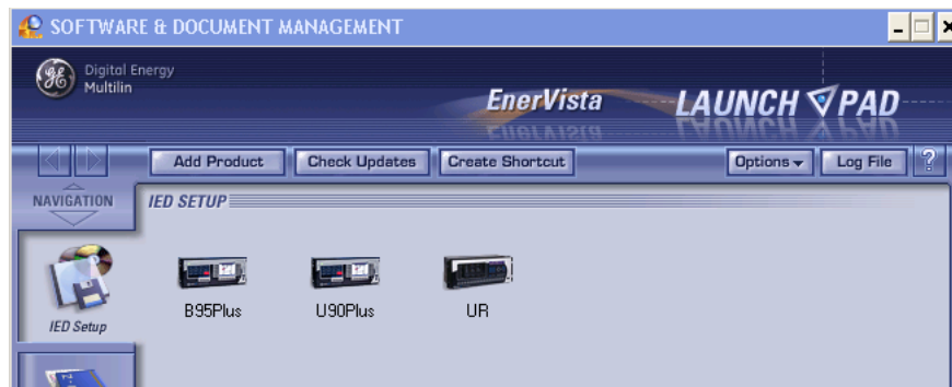
Figure 3-57: UR device added to Launchpad window
