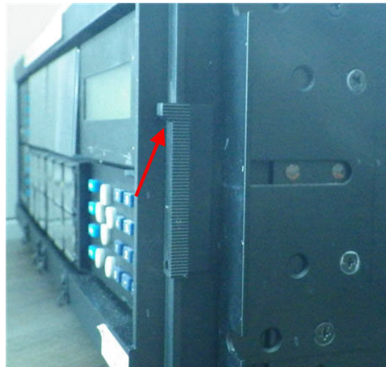
Figure 10-15: Lift latch on basic front panel to open
