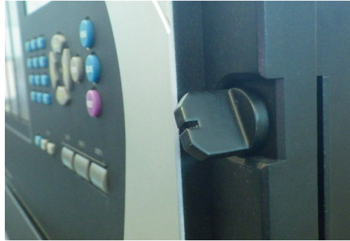
Figure 10-15: Lift latch on basic front panel to open
