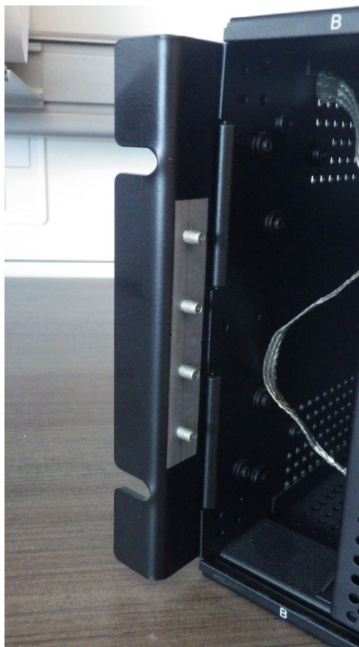
Figure 10-21: Attach mounting bracket on left side (enhanced front panel shown; no power supply module in first slot)
