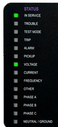
Figure 4-52: Example of LEDs on graphical front panel
