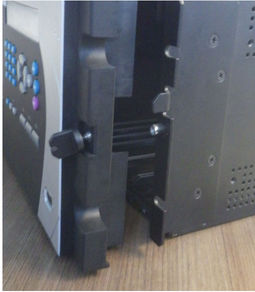
Figure 10-17: Remove basic front panel mounting bracket on right side
