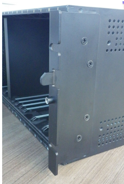
Figure 10-22: Attach mounting bracket to relay on right side
