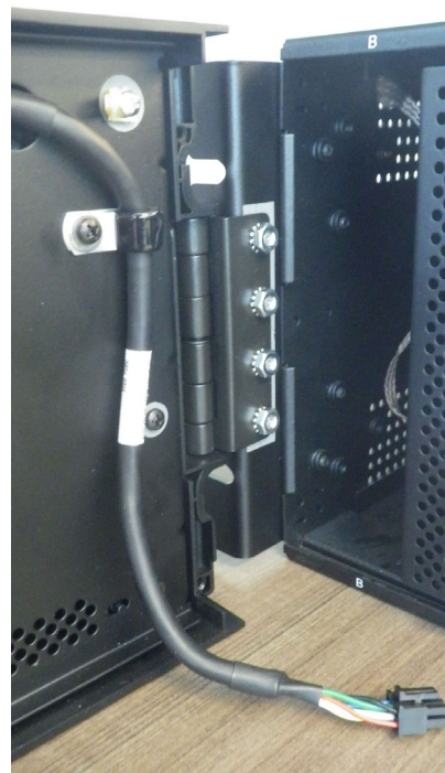
Figure 10-23: Attach to left mounting bracket inside relay
