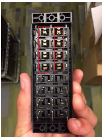
Figure 22: Terminal block with eight shorting clips
