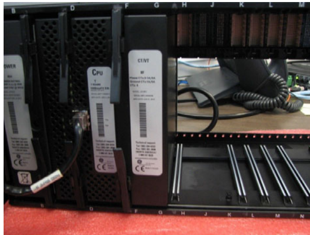
Figure 28: Push levers in to insert module fully
