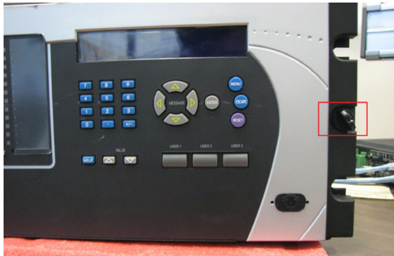
Figure 20: Open the front panel (enhanced front panel shown)
