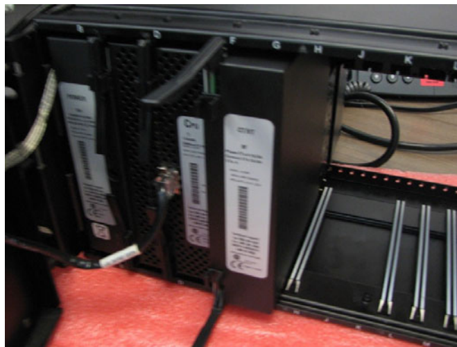
Figure 21: Pull module levers out
