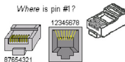
FIGURE QS-1: Pin Layout for a RJ45 Ethernet Straight-through Cable
