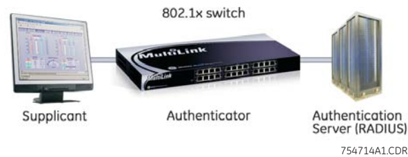
FIGURE 7-1: 802.1x network components
