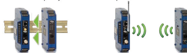
Expansion modules connected via backplane
