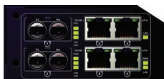
4 - 10/100 Mbit Copper RJ45 Ports 2 - 100 Mbit ST, or SC Fiber Ports
