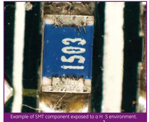
Example of SMT component exposed to a H 2 S environment.
